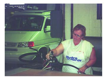
Major RV OEM Using a Portable HYDRA 55 to Spray M6187 to bond wood to foam for headliners and (below) foam and fabric to a metal seat boxspring
