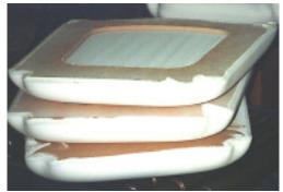
In an extremely demanding application for a water-based adhesive, M6187 is used to bond 3 pieces of different density foams to the edge of a wood seat frame.
