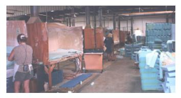
Fabrication stations with gun drop panels off of master tote system
