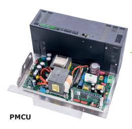
Compact Power Management Control Unit (PMCU) which unifies the central control unit, internal/external communication (CAN-Bus/ Ethernet) and power interfaces between power inverter and battery (DC-DC-converter, isolation) with regard to functional safety.
