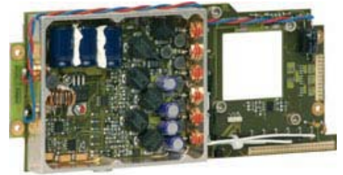
Design engineers may decide to opt for a custom power supply to minimise EMI. A low-EMI embedded power system is pictured.
