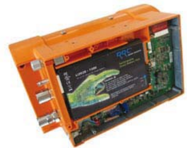
This embedded power management system is designed for use with a respirator.
