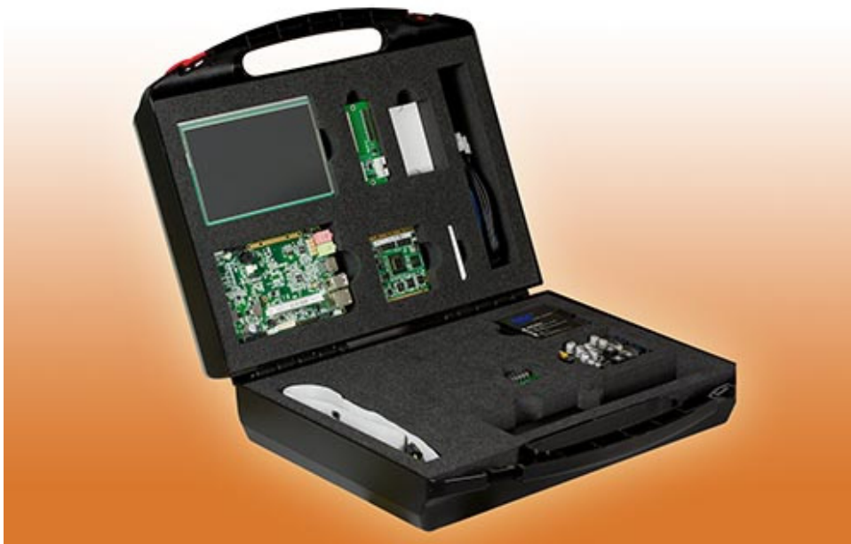
Fig 4: Mobility Starter Kit with all necessary hardware (SBM3, RCC battery pack, Computer-on-Module, carrier board, display and cable set) for fast evaluation
