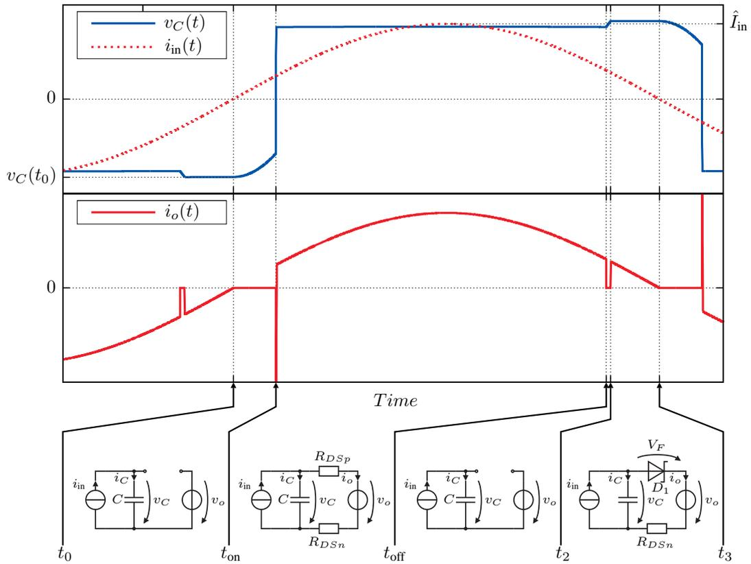
Figure 5. One half period of the rectifier input voltage  $v_C(t)$  and the output current  $i_o(t)$  at sinusoidal input current  $i_{in}(t)$ .
