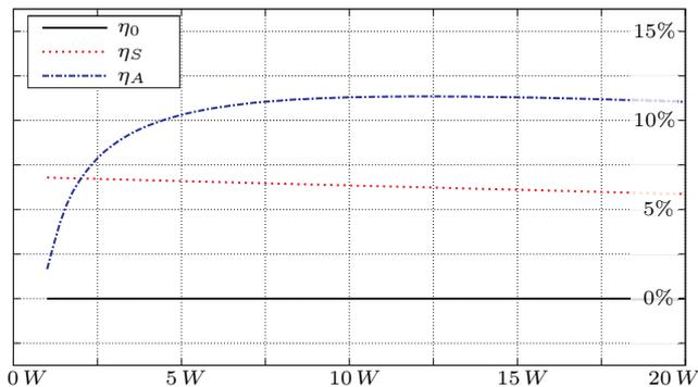
Figure 7. Efficiency Improvement normalized to  $\eta_0$  which is the efficiency with a passive rectifier.  $\eta_S$  is the efficiency with a semi-active rectifier (lower MOSFETs are self-driven and only the body diodes of the upper MOSFETs are active) and  $\eta_A$  is the efficiency with the proposed full-synchronous rectifier
