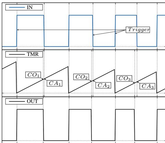
Figure 3. Input and output signal at the MCU with corresponding timer. The second timer works similar, but with an phase shift of one half period.
