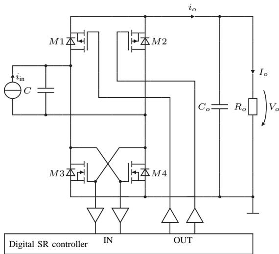
Figure 2. Proposed synchronous full-bridge rectifier
