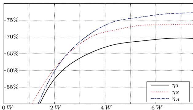
Figure 8. Efficiency measurements.  $\eta_0$  is the efficiency with a passive rectifier.  $\eta_S$  is the efficiency with a semi-active rectifier (lower MOSFETs are self-driven and only the body diodes of the upper MOSFETs are active) and  $\eta_A$  is the efficiency with the proposed full-synchronous rectifier
