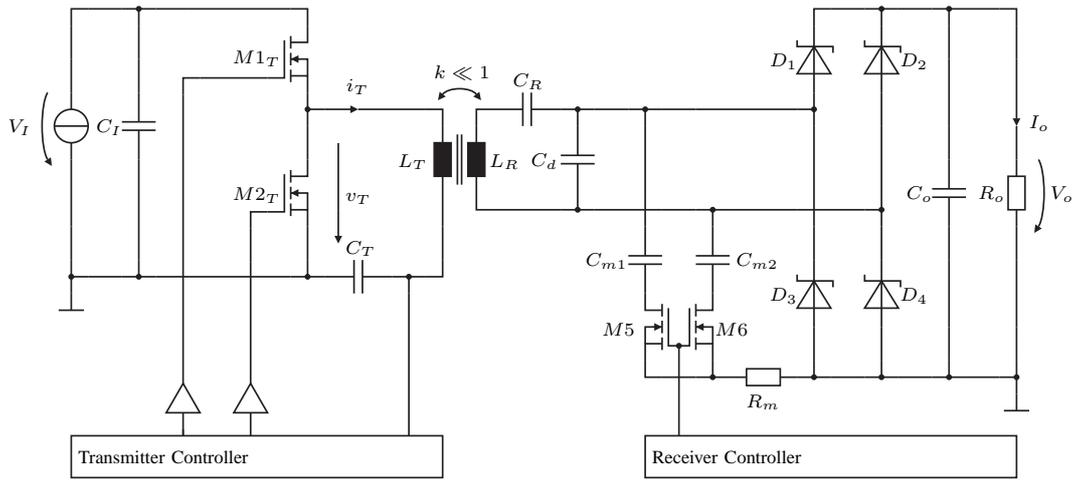
Figure 1. Qi-compliant WPT circuit using an A1 transmitter design as specified in the WPC standard [4]
