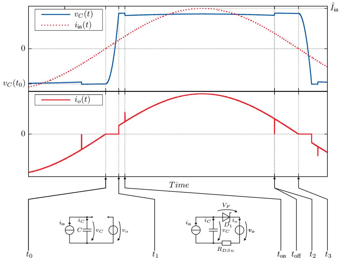
Figure 6. One half period of the rectifier input voltage  $v_C(t)$  and the output current  $i_o(t)$  at sinusoidal input current  $i_{in}(t)$ .
