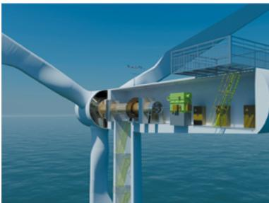
Picture: One SMPS per rotor blade, i.e. three SMPS for the complete pitch control of a wind turbine generator system.
