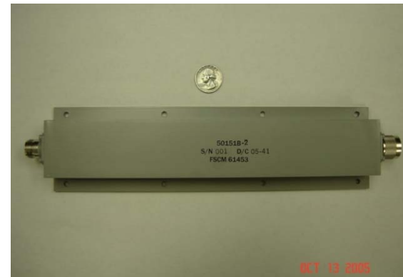
→ Low-Loss High Rejection Bandstop Filter 50151B (10/05)
