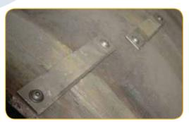
Figure 3: Obstacle plates attached to the drum
