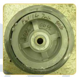
Figure 4: Typical Failure during an Obstacle Test
