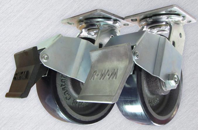
The RWM Installable Cam Wheel Brake or "ICWB" for short is one of the best brakes for 2" wide wheels in the industry and is the recommended upgrade over most other 2" brake options. This brake is a great fit for medium duty casters, especially Kingpinless ™, and offers exceptional performance to lock the product in place. The pedal rotates a metal pad, which locks the wheel in place.
