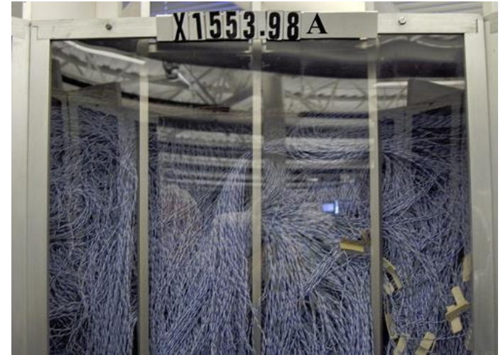
Cray 1A Serial Number 6 Computer History Museum 80 MHz cycle time Quite the cable management problem
