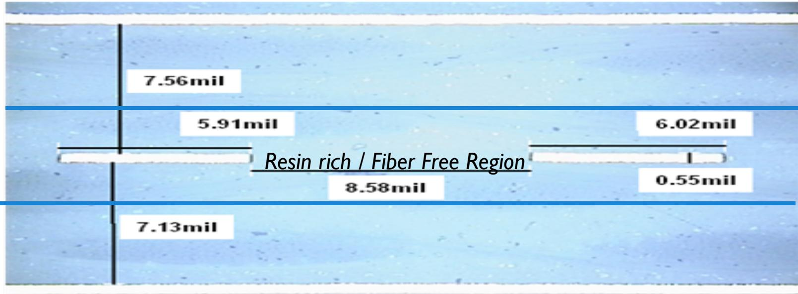
To correctly model differential trace geometries, anisotropic layering must be modeled. Resin/Epoxy/Polymer regions are always lower Dk than mixed dielectric regions. Laminate weave skew is identified and bounded through measurements and then incorporated into channel models as a post process step.
