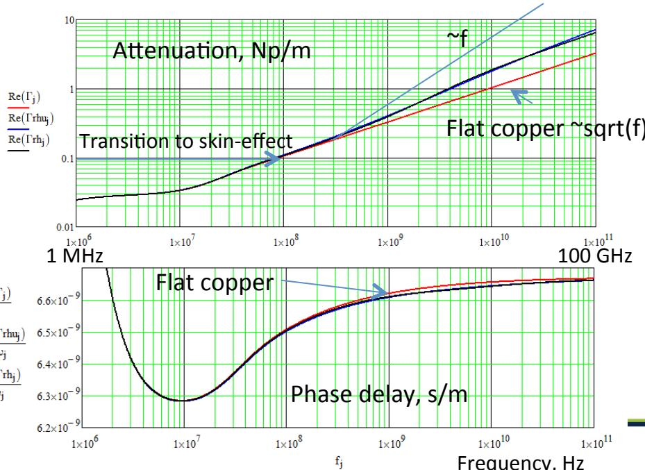
Roughness has a large impact on loss.
