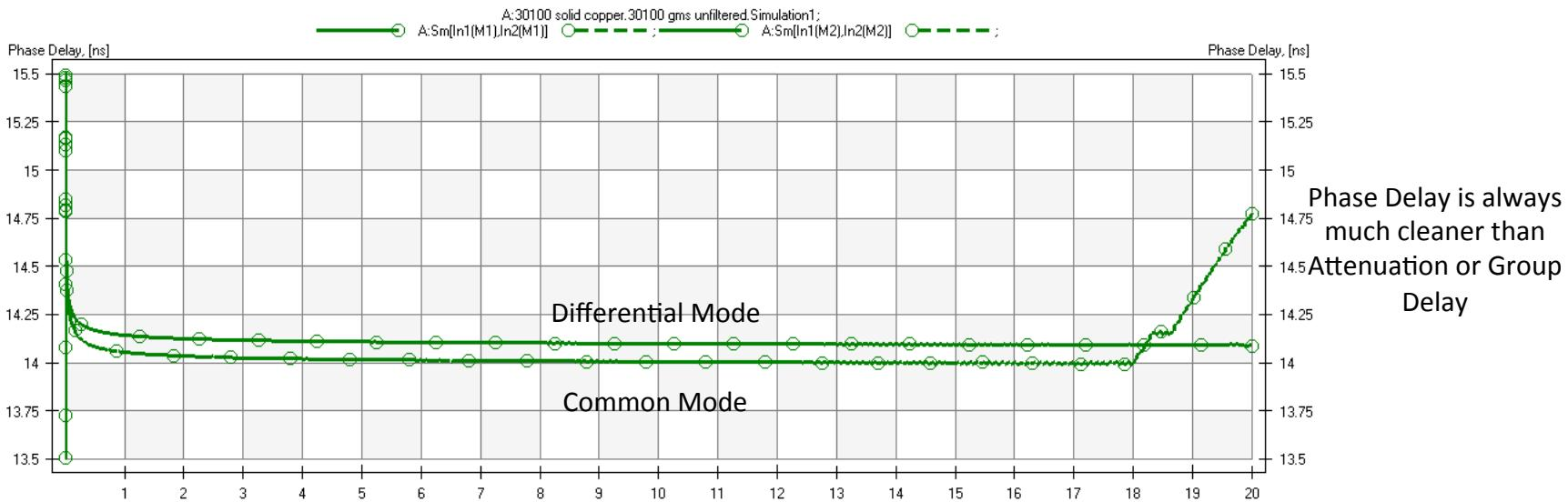
Mode separation occurs when dielectric is not uniform when working with differential conductors. The position of Differential Mode vs Common Mode provides information on where the difference occurs. Faster Common Mode indicates common mode fields are exposed to a lower Dk dielectric.
