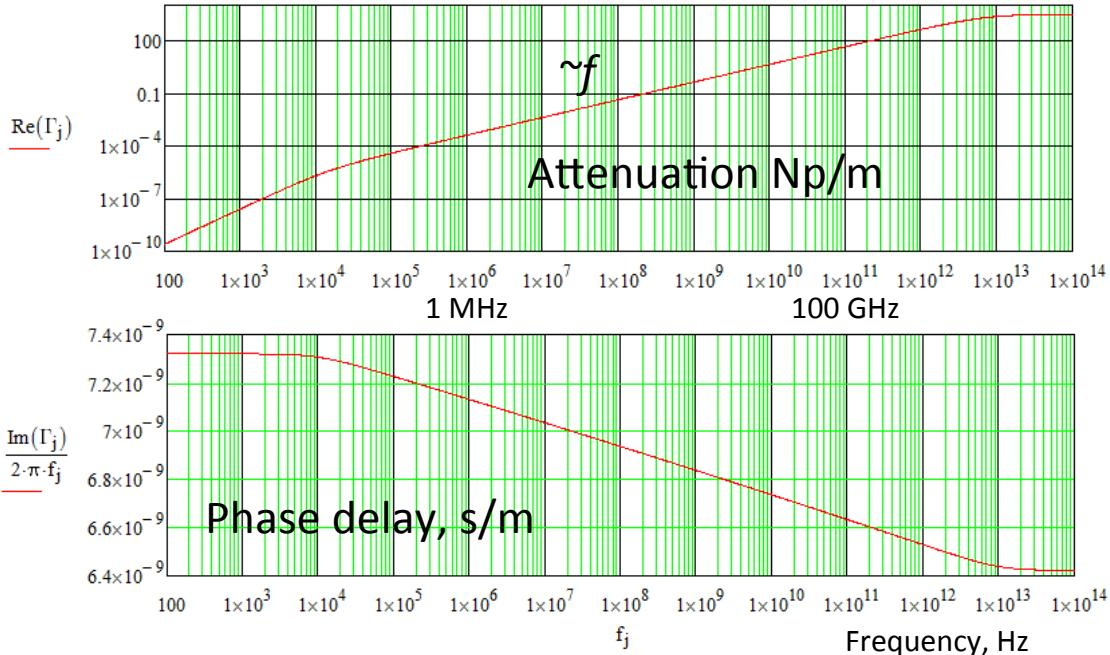
Both attenuation and phase delay provide the same information regarding the dielectric loss.
