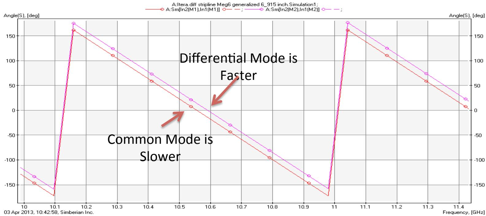
Mode separation due to layered anisotropy of epoxy and fiber rich areas in laminate system
