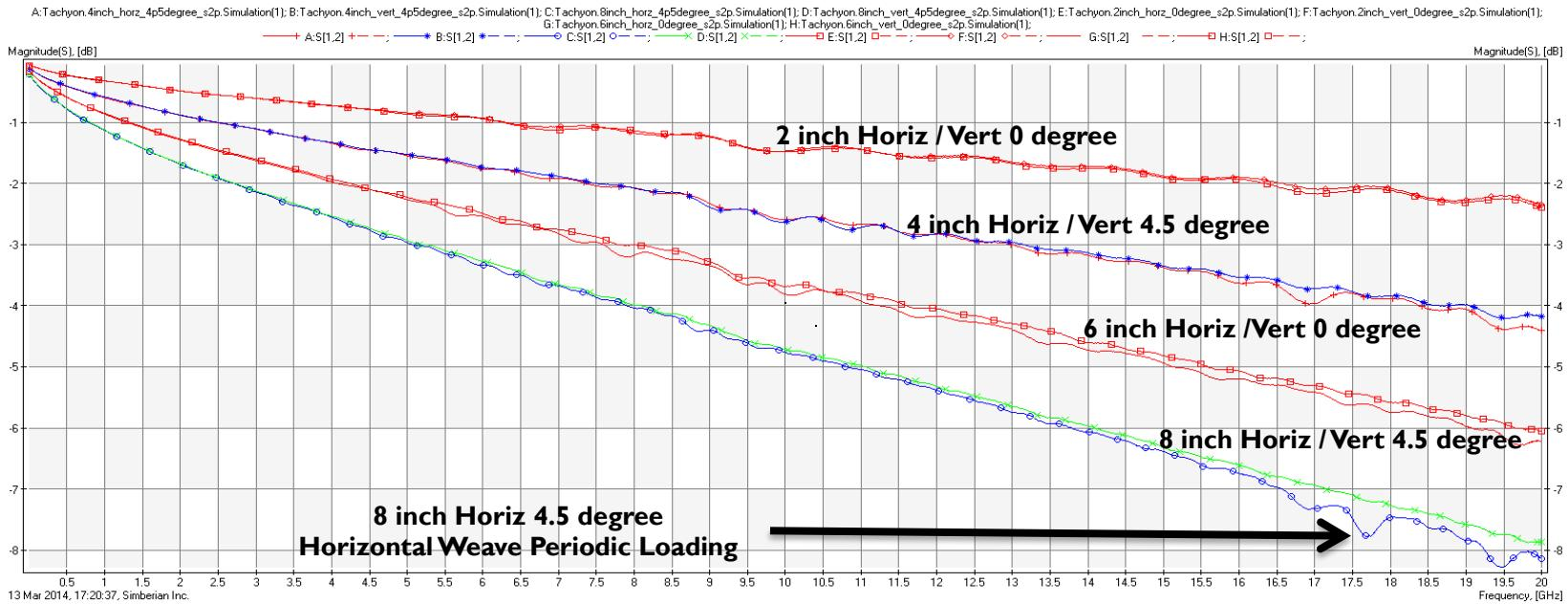
Variation of Dk in horizontal weave direction is discerned by 4.5 degree periodic weave loading, which causes a  $\frac{1}{2}$  wave resonance at  $\frac{1}{2}$  the crossing frequency
