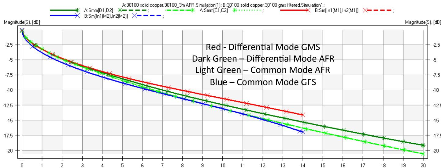
GMS-parameter method is designed to remove losses due to impedance mismatch by normalizing to a perfectly matched condition at every frequency point.
