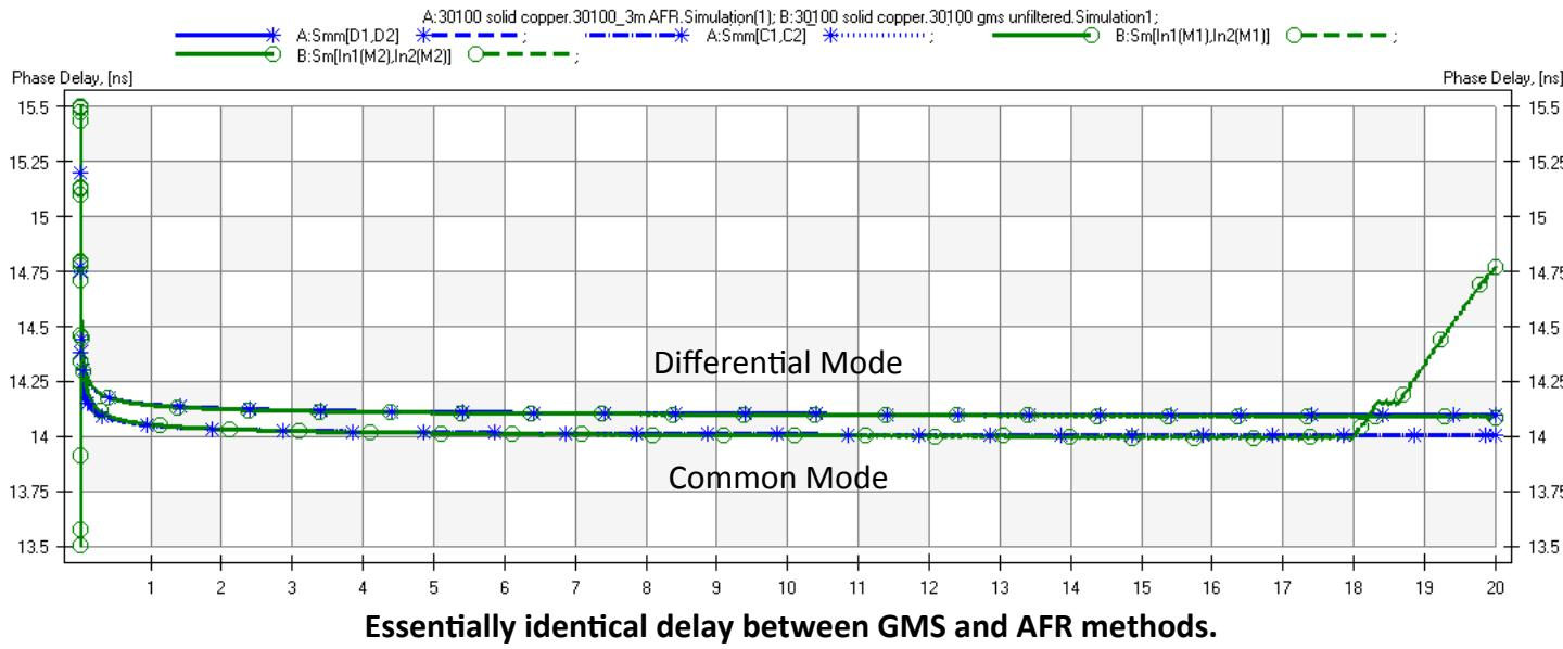
Phase or Phase delay is generally the most stable method for identifying dielectric properties.
