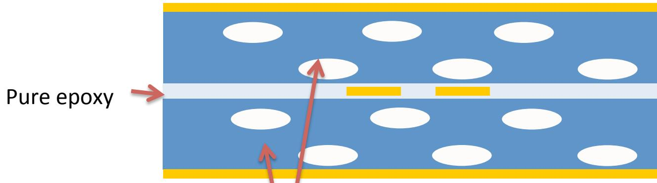
Difference between epoxy Er and Average Er results in separation of common and differential propagation modes.
