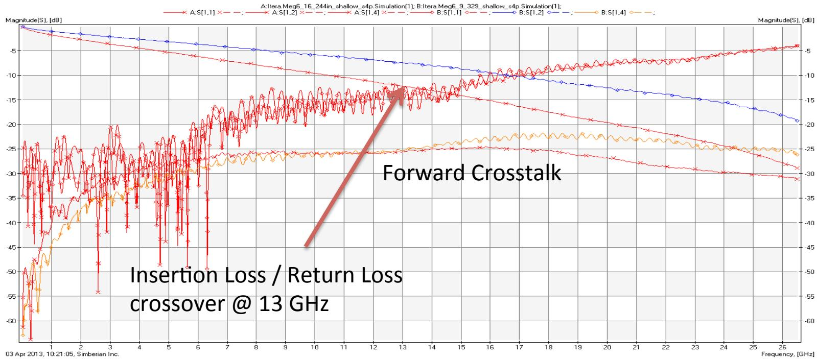
Measured data is often limited by Signal-to-Noise ratio at the insertion loss / return loss crossover point. But even this data can produce good model correlation if parameters are extracted between DC and 13 GHz.
