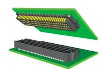
SEAM/SEAF High Speed/High Density Array Pitch: .050" (1,27 mm) Total Positions: 40 - 150 Stack Height (mm): 7-17.5 Performance: Single Ended - 12.5 GHz (7 mm Stack Height) Differential Pair - 13 GHz (7 mm Stack Height) **Orientation:** Vertical and Right Angle
