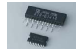
ACアダプタ専用高性能IC STR-E1414/SPF9140
