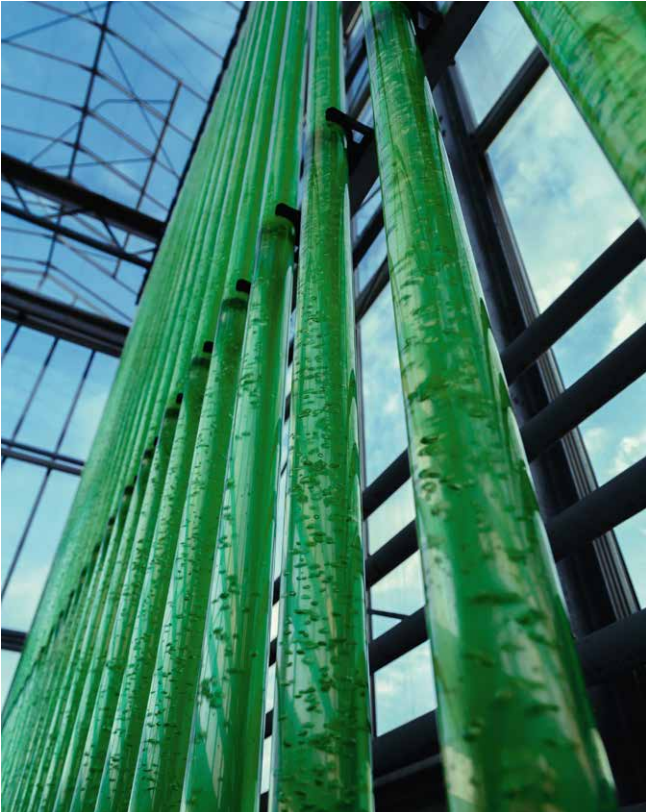
Tubular Glass Photobioreactors (PBR) located at ecoduna, Austria
