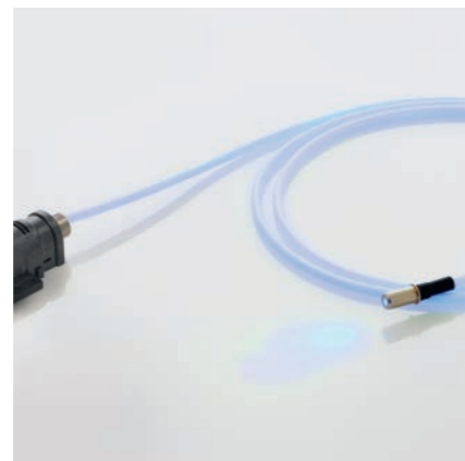
HelioLine glass fibers are powered by a separate light source. There are two main advantages: A: The light source can be placed away from the point where the light is emitted. B: The glass fiber does not carry any electrical power.
