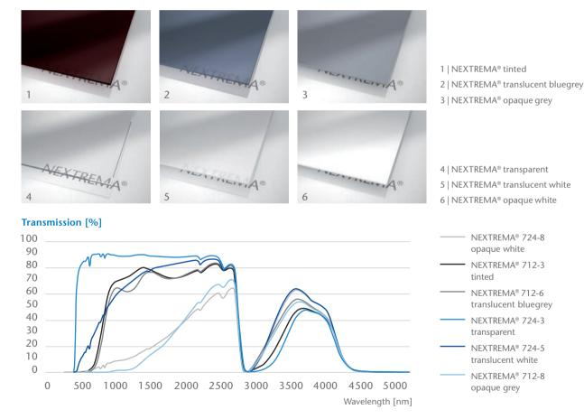
This graph is based on data from individual measurements. Deviations may result from manufacturing process. Internal transmissions graph of different ceramization status with sample thickness of approximately 4 mm.
