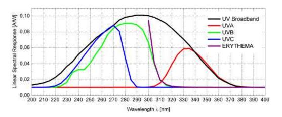
The graph assigns the filtered photodiode's spectral response to an individual wavelength. The following table extracts the most important specifications.
