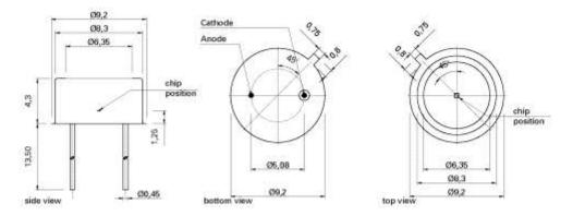
Selection Code "5" (photodiodes without filters)  $\rightarrow$  TO5 Ni plated housing, 9.2 mm diameter, 4.3 mm height, two gold plated pins (Anode grounded and Cathode isolated).
