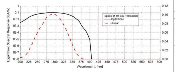
The curve's maximum is at approximately 300nm. The response falls down to 10% of maximum at 215nm, (UVC edge) and 365nm, (UVA edge). Unfiltered SiC can be used for any UV measurements where the whole UV band needs to be measured or a quasi monochromatic UV source (such as low pressure lamps) is controlled.
