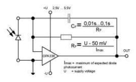
The adjacent design gives an example of a simple amplifier circuit. At the left side the photodiode is shown. The upper connection is the Cathode (isolated pin of the photodiode) and the lower connection is the Anode (usually grounded pin of the photodiode).
