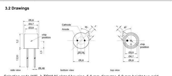
Selection code "18"  $\rightarrow$  TO18 Ni plated housing, 5.6 mm diameter, 5.2 mm height two gold plated pins (Anode grounded and Cathode isolated).
