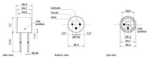
Selection code "18ISO90"  $\rightarrow$  TO18 Ni plated housing, 5.6 mm diameter, 5.2 mm height three gold plated pins (Anode and Cathode isolated, additional third pin for optional grounding of the body).
