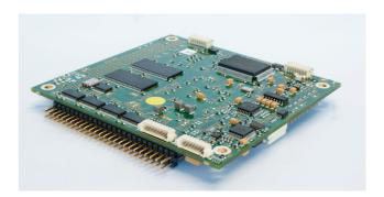
The XA270 has been designed using state of the art RISC technology using Intel®'s XScale® XA270® high performance, low-power, high-integration systems-on-a-chip (SOC) processor designed for low power portable computing applications. This concept enables the board to run industry standard operating systems and applications, thereby reducing the development time for the user.
