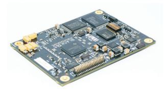
BLACK365 combines the power of the Texas Instruments DM365 processor with a comprehensive set of peripherals optimized for high functionality, low power and small form factor. This low power credit card size board is ARM9® based and is designed for high performance digital media applications and supports a range of encode, decode, and video quality operations.
