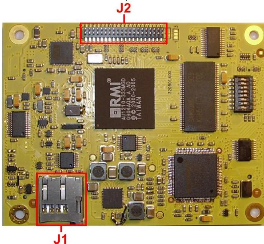
**FIGURE E1 - YELLOW1210 CONNECTOR POSITIONS – TOP SIDE**
