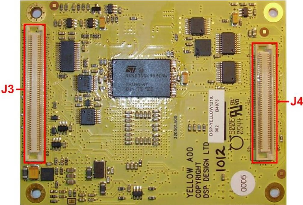
FIGURE E2 - YELLOW1210 CONNECTOR POSITIONS – BOTTOM SIDE
