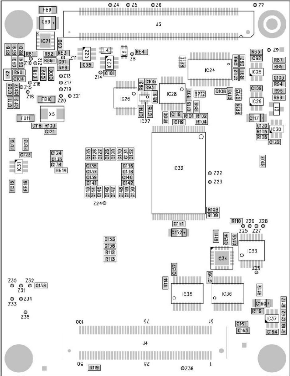
FIGURE B2 - YELLOW1210 COMPONENT PLACEMENT DIAGRAM – BOTTOM SIDE
