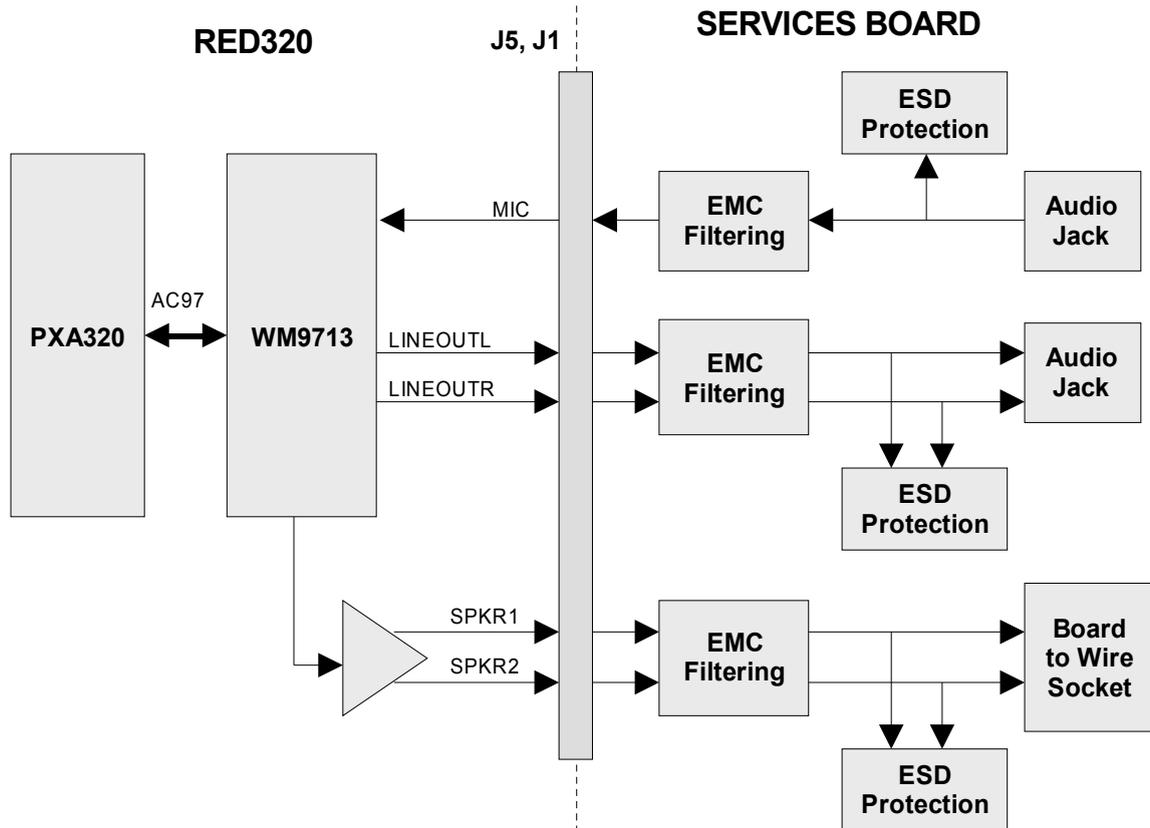
**FIGURE 7 - YELLOW1210 AND SERVICES BOARD AUDIO BLOCK DIAGRAM**
