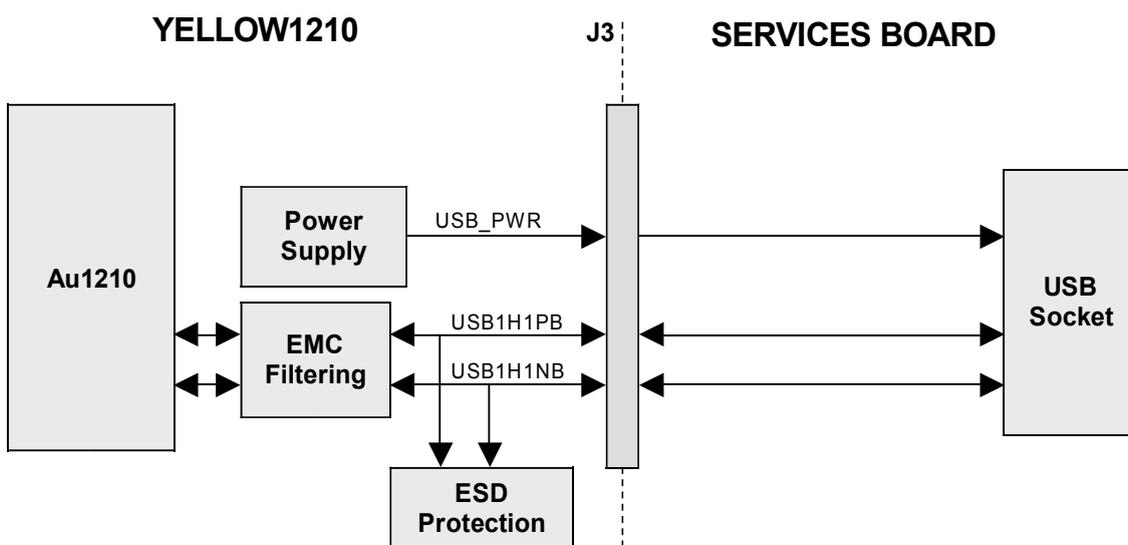
**FIGURE 5 - YELLOW1210 AND SERVICES BOARD USB HOST BLOCK DIAGRAM**
