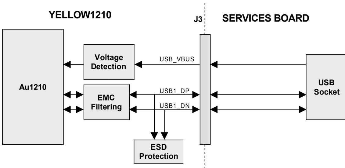
**FIGURE 6 - YELLOW1210 AND SERVICES BOARD USB CLIENT BLOCK DIAGRAM**
