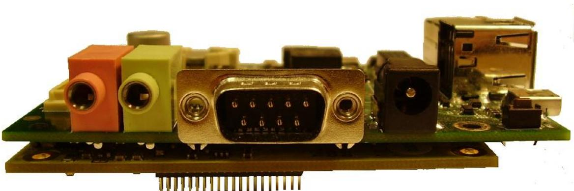
**FIGURE F3 - YELLOW1210 AND REDCONN CONNECTED BACK-TO-BACK**
