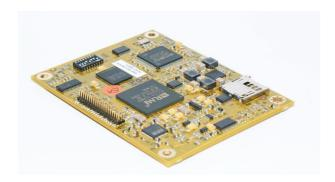
YELLOW1210 is a high performance credit-card size single board computer optimized for use in embedded projects. YELLOW1210 combines the power of the Broadcom® Alchemy™ Au1210™ processor with a carefully selected set of peripherals optimized for high functionality, low power and small form factor. DSP Design has engineered the high risk elements of the system. You receive a fully tested module loaded with an operating system ready for your integration.
