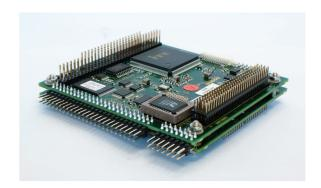
The TP600 is based on the AMD Geode™ LX800 @ 0.9W CPU providing a highly integrated, Pentium-Class processor module. Its high speed and extremely low power consumption make it ideal for use in processor intensive applications requiring rugged construction and short time to market.
