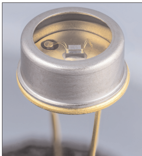
Encapsulated UVC LED for water disinfection. ©FBH/Schurian.co.
