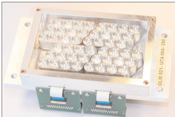
Water-cooled UV LED radiant source 4xOLM-021a. ©OSA Opto Light GmbH.
