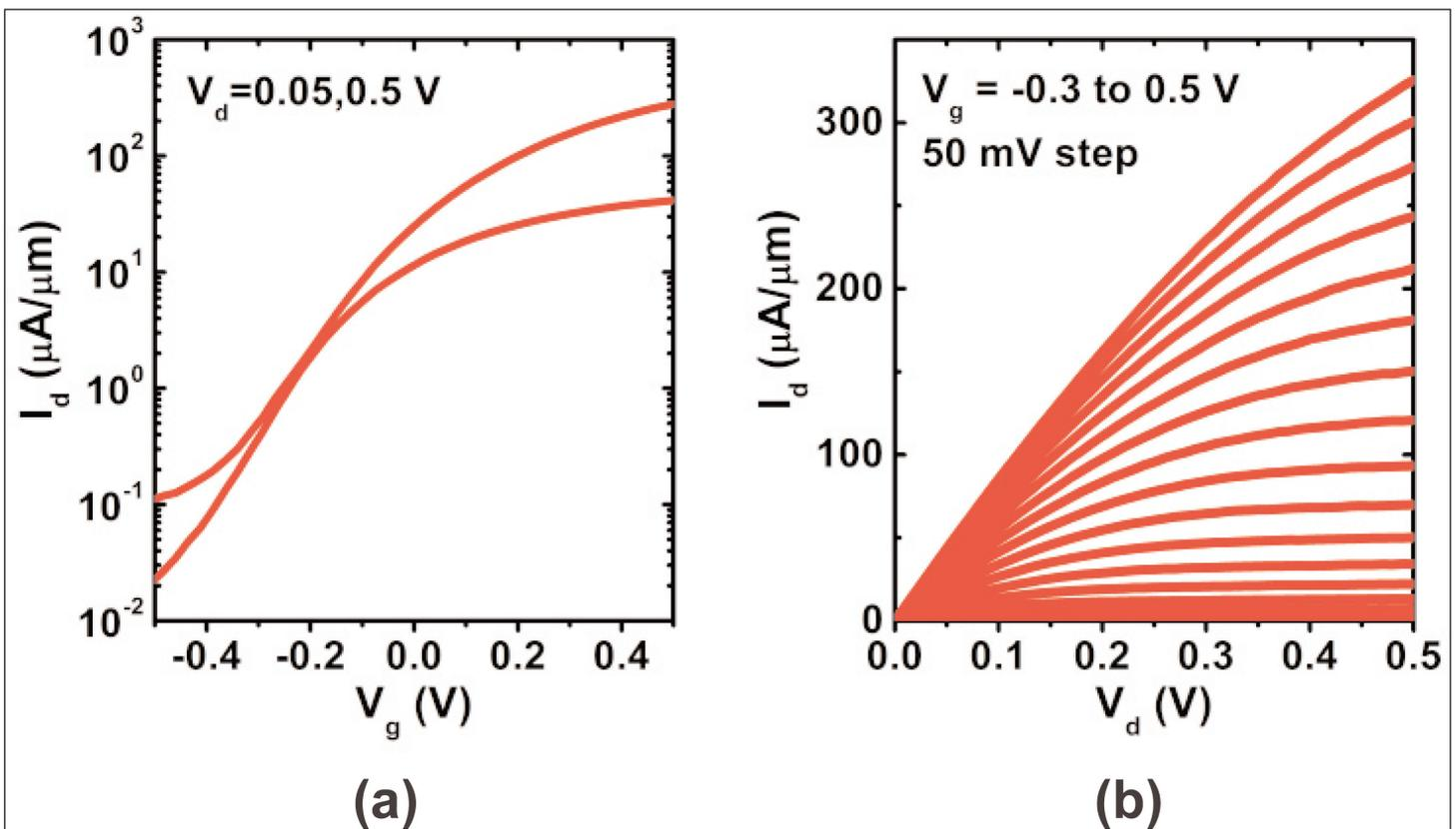
**Figure 2. (a) Drain current versus gate voltage ( $I_d$ - $V_g$ ) of typical device at 0.5V and 0.05V drain bias ( $V_d$ ). (b) Drain current and voltage of same device with  $V_g = -0.25$  V to 0.50V in steps of 50mV.**
