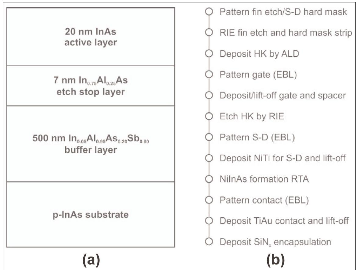
**Figure 1. (a) The layer structure that was used, showing the pseudomorphic InAlAs etch stop layer and (b) the process flow for fabrication of InAs finFETs, starting with the first step after wafer growth.**
