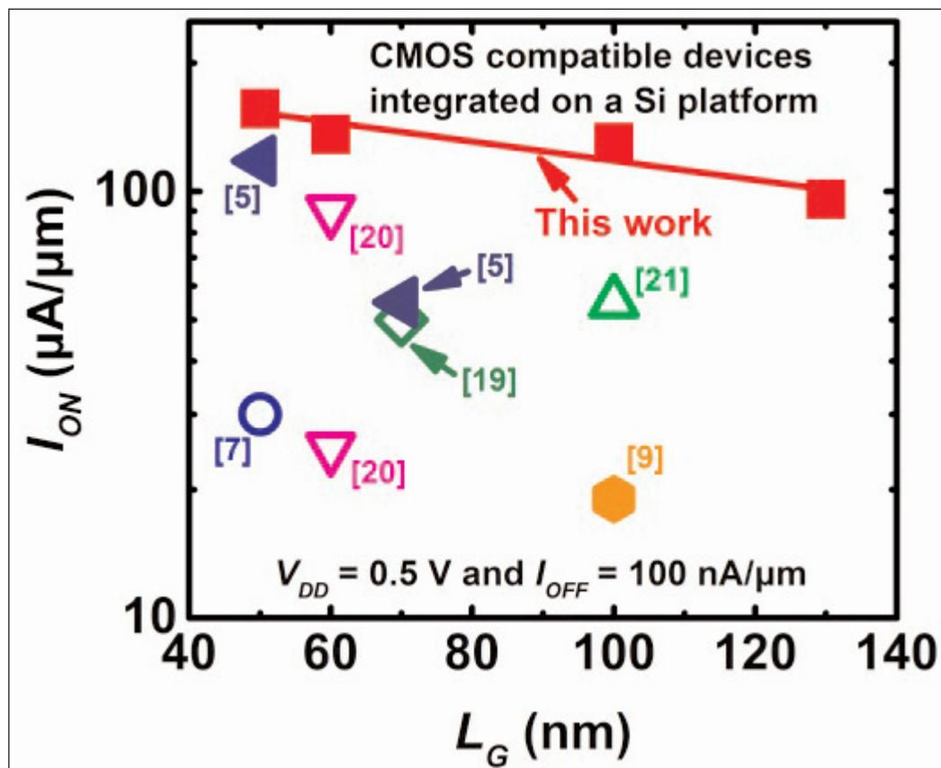
**Figure 4.**  $I_{\text{ON}}$  versus  $L_G$  benchmark of CMOS-compatible InGaAs FETs integrated on silicon platform.  $I_{\text{ON}}$  values are extracted at 0.5V operating voltage and an  $I_{\text{OFF}}$  of 100nA/ $\mu\text{m}$ .
