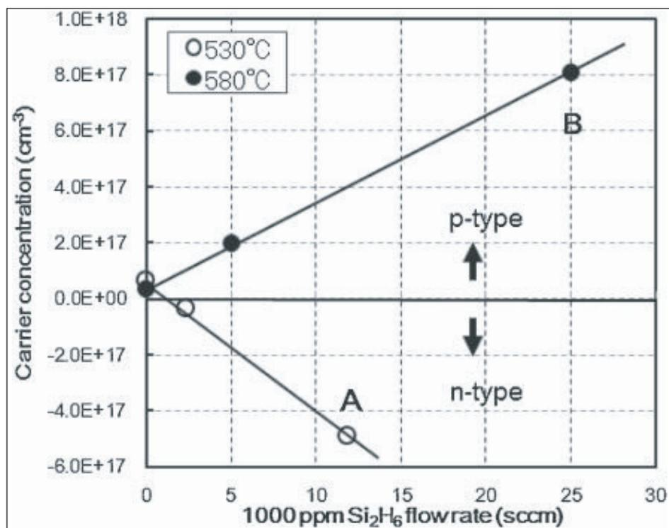
Figure 1. Si<sub>2</sub>H<sub>6</sub> flow rate dependence of carrier concentration in silicon-doped GaAsSb layers.
