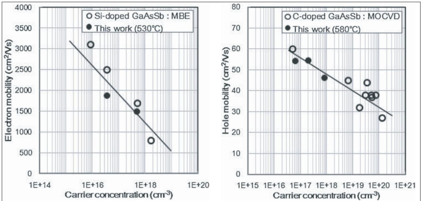
**Figure 2. (a) Relationship between electron mobility and electron carrier concentration in Si-doped GaAsSb layers grown at 530°C, compared with MBE GaAsSb:Si. (b) Relationship between hole mobility and hole carrier concentration in Si-doped GaAsSb layers grown at 580°C, compared with MBE GaAsSb:C.**
