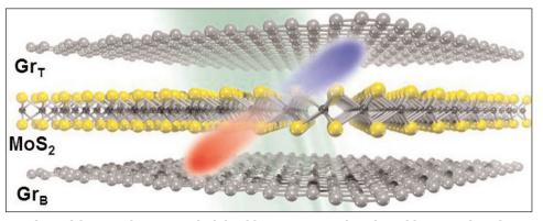
Device with  $MoS_2$  layer sandwiched between top (GrT) and bottom (GrB) graphene layers. Light (green ray) is absorbed and converted into electric current. When light is absorbed by the device, electrons (blue) jump into a higher energy state and holes (red) are generated in the  $MoS_2$  layer. Motion of holes and electrons created by the difference in electronic potential between the GrT- $MoS_2$  and the GrB- $MoS_2$  junctions generates the electric current.
