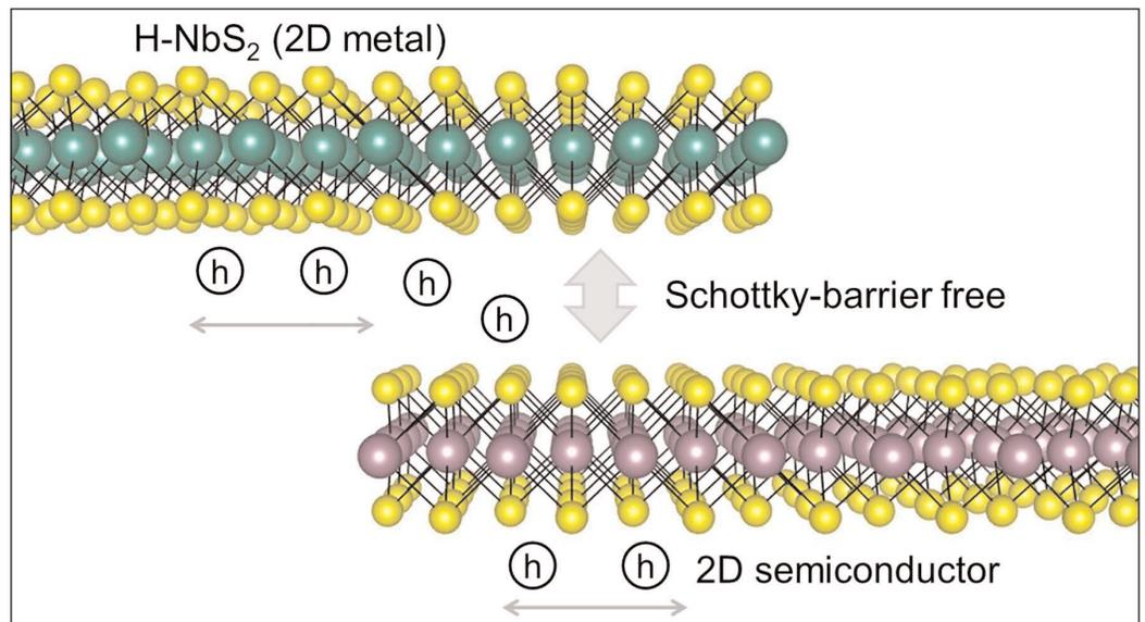
**Using 2D metal as contact for 2D semiconductor allows Schottky barrier to be tuned, due to the weak Fermi level pinning at the junction caused by the suppression of metal-induced gap states. Schematic illustrates that 2D H-NbS<sub>2</sub> can form a Schottky-barrier-free contact with 2D semiconductor for hole transport.**
