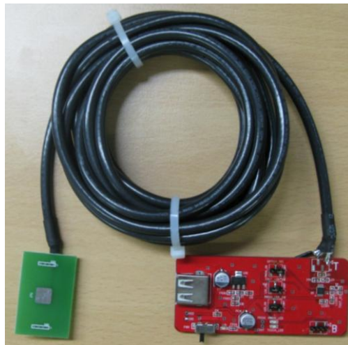
Figure 27. 3 meter shield cable between a touch electrode and the ATA5101
