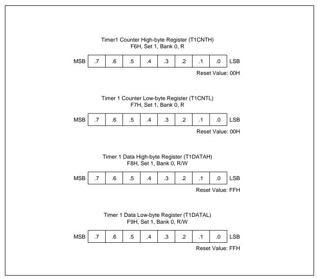
Figure 11-5. Timer 1 Registers (T1CNTH, T1CNTL, T1DATAH, T1DATAL)
