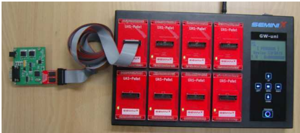
Connect GW-uni2 plus to User board via UAS-Pellet2 Adapter Cable
