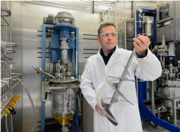
The glass and stainless steel test stand for stirring installed in a hood.
