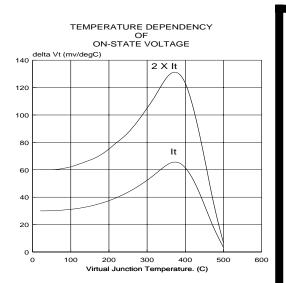
Fig.4 The charge in on-state voltage per degree Celsius is shown as a complex function of temperature. Two current levels are plotted.
