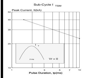
Fig. 2  $I_{\text{ISM}}$  as represented through the sub-cycle range. This curve is used to coordinate with fuse let-thru current.
