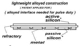
\* both silicon thicknesses matched for zero bow
