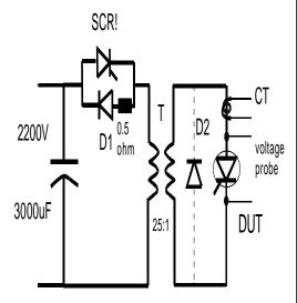
Fig.3 Type of laboratory circuit used to verify or establish ratings for  ${\rm I}_{_{\rm IM}}$  and pulse power
