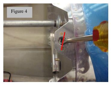
Reinstall your panel and check that all fasteners lock properly; are not too tight or too loose. If you are installing a large panel or engine cowling, place a piece of masking tape at each fastener location and mark ½, 1, or 2 turns to loosen or tighten fasteners. ½ turn is the equivalent of .015 adjustment; a full turn is .030; or the same as if you exchanged studs for proper fit.
