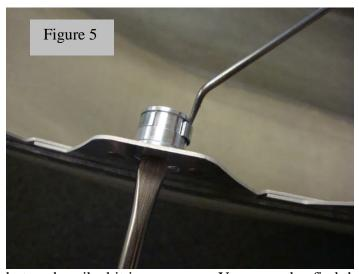
In Figure 5, with the outer panel removed, insert the curved pick tool into the rear groove to lift the locking clip and use a standard screwdriver to turn the insert accordingly. Remove the pick and check that the insert is locked.
