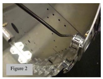
Before you begin installation, note the black anti-lock pin installed at the back of the receptacle (Figure 1). This pin has one function: to allow for the initial adjustment setting. You will note that the inner member is free to rotate. It is important to note the orientation of the pin as you mount the receptacle. Obviously, it can be mounted orientated in two directions. You want to mount the receptacle such that the pin, better worded, the locking clip "tang" is accessible as noted in
