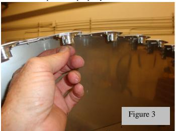
place the panel in position and lock the fastener into receptacle. (If the insert is too far inside of the receptacle barrel, you may not be able to lock the fastener. Simply position the outward towards insert the surface). Once locked, continue to turn the fastener as if it is a simple machine screw. This will draw the fastener to the proper clamped and locked position which is approximately .020 from fully bound (clamped).
