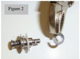
To install: Bend retainer open enough (Figure 2) to rotate around stud pin (Figure 3)
