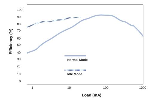
Consumer with 10mA load:-70% @ Normal =  $\sim$ 13mA 90% @ Idle =  $\sim$ 11mA Saving  $\sim$ 2mA
