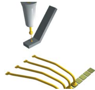
FAB formation during wire bonding process
