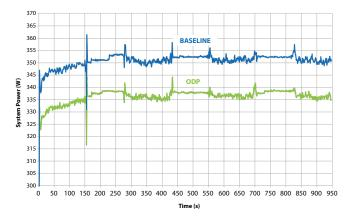
Figure 2: Measured power savings in a server configured with sixteen 16GB DDR3 EcoMemory modules vs sixteen standard RDIMMs
