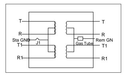
Figure 1: P30051 4-Wire Card Schematic
