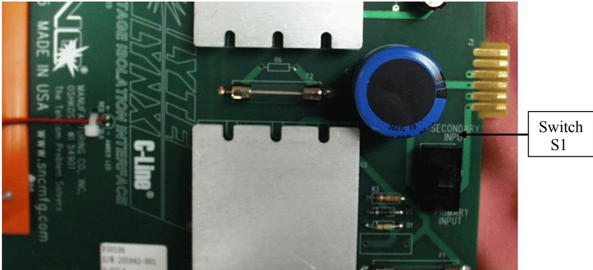
FIGURE 2: P30106 - 120VAC/130VDC to 48VDC Power Supply
