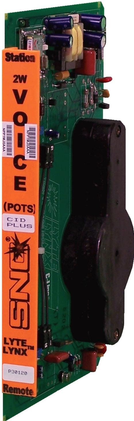
substations and similar locations where high voltage isolation is required on the incoming copper phone pairs to protect the network from harm and to provide a personnel safety barrier against voltages. This specifically includes protection from longitudinal voltage surges and Ground Potential Rise (GPR) surges that may occur during power system faults.
