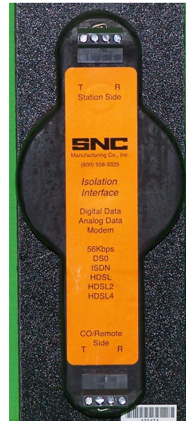
P31042 2-Wire 56kbs Data Isolation
