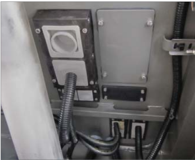
KEL-JUMBO 2 - Page 34 / KEL 24|x - Page 18 Routing of conduits and large cables between vehicle body and chassis
