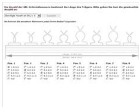
Example 2: Clamp assembly 8-piece with integrated strain relief and different SKL shield clamps
