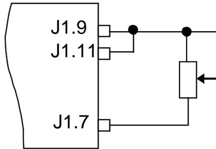
**Figure 4-6** Programming Output Voltage using an External Resistor
