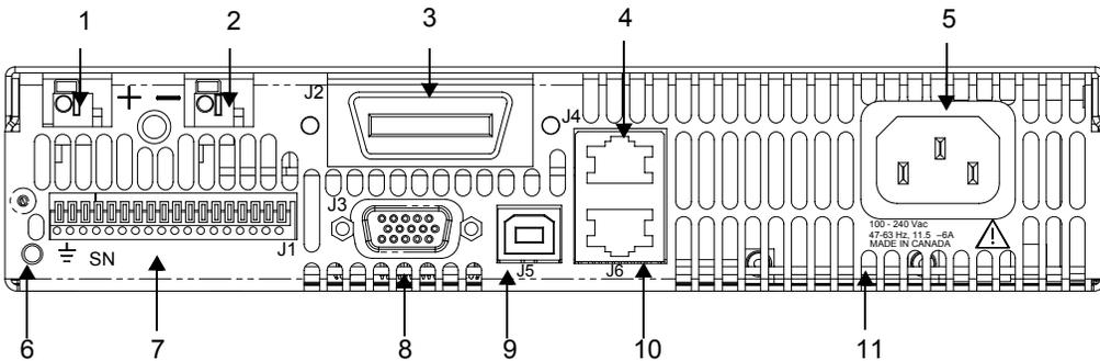
Figure 1-5 Rear Panel: 300 V to 600 V Models
