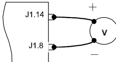
**Figure 4-9** Current Readback Using APG Connector J1
