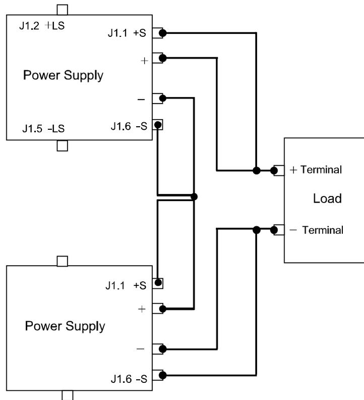
Figure 3-7 Load Connections in Remote Sensing Mode
