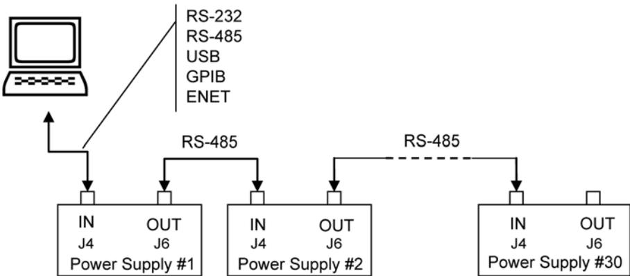
Figure 5-13 Multi Power Supply Connection to RS-485 Bus
