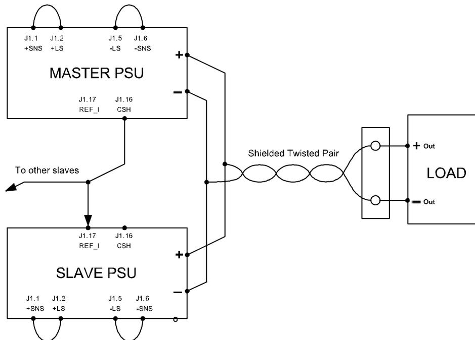
Figure 3-8 Load Connections in Local Sensing Mode
