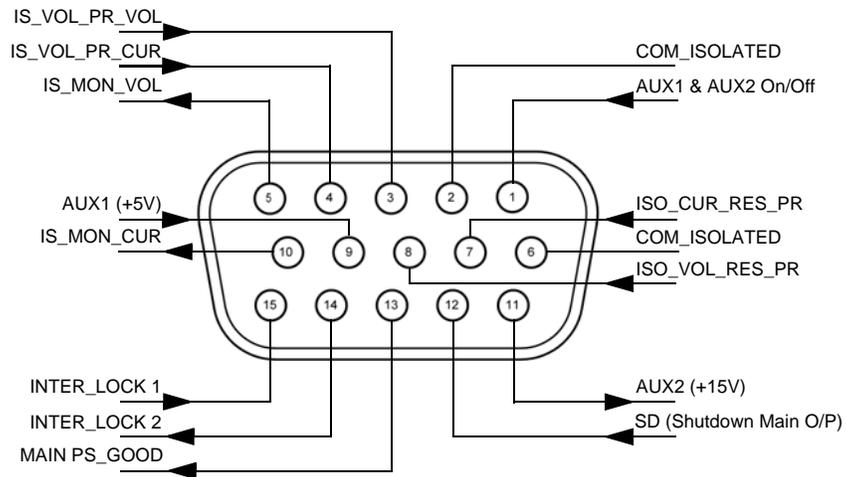
**Figure 4-10** AUX Output and ISOL Connector Pinout
