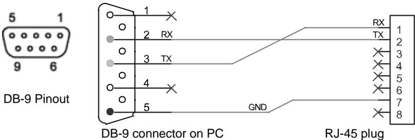
Figure 5-2 RS-232 Communication Cable with DB-9 Pinout
