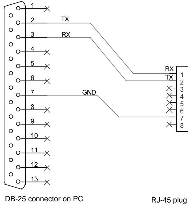
**Figure 5-4** RS-232 Communication Cable with DB-25 Pinout
