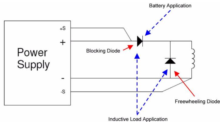
**Figure 2-2** Diode Placement
