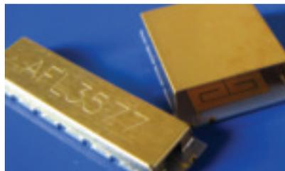
The third option leaves packaging up to the customer. Either the next level of assembly provides the RF shielding for the filter or the customer can have its own cover integrated.
