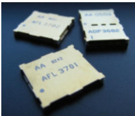
A second option is the attachment of an integral metal cover to the filter. Typically, the cover will have tabs that fit into ground vias along the perimeter of the part and a high-temperature solder will be used for the assembly.
