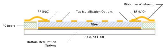
The above illustration demonstrates the mounting of a typical chip and wire filter. The circuit is relieved to accommodate the filter. The bottom surface of the part is attached directly to the system ground plane using conductive epoxy. Wire or ribbon bonds are launched from the circuit to the filter I/O pad. In a typical application a channelized housing would sit over the filter to provide adequate RF shielding.
