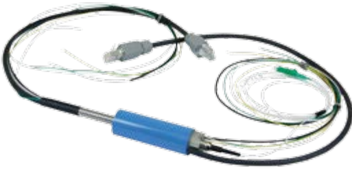
SPINNER FORJ 1.14 with slipring: The perfect match for cable-suspended camera system
