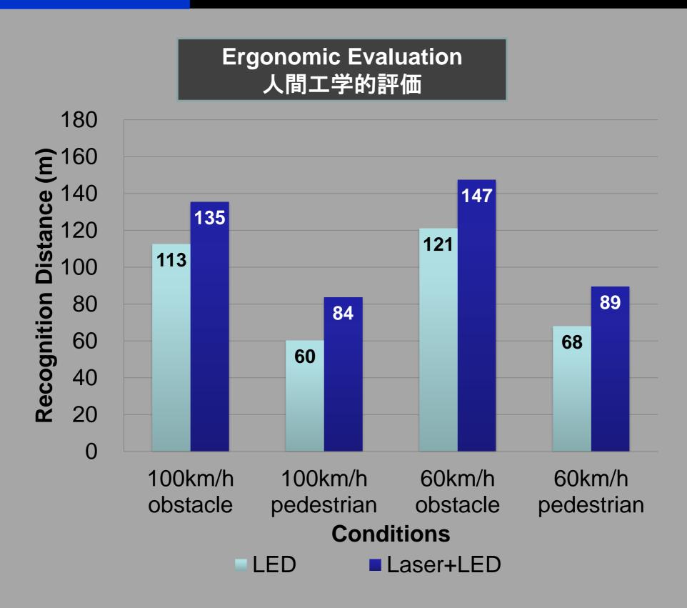
The recognition distance of Laser +LED lamp is 20~30m further. 20~30m手前で気づくことができます
