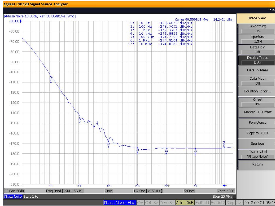
Figure 26: 100MHz Crystal Oscillator Measured on Agilent E5052B (Corr_4000)
