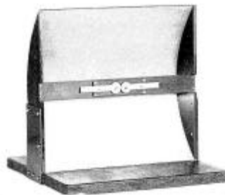
Figure 1-3 Dipole oscillator after Ludenia placed in a parabolic mirror to increase efficiency (1929).
