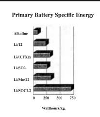
The Lithium Thionyl Chloride battery has the highest energy density of production primary batteries. Just as with other chemistries such as lithium ion, lithium thyonyl shloride performance is manufacturer dependent. Tadiran's have the highest energy density, voltage and temperature range.
